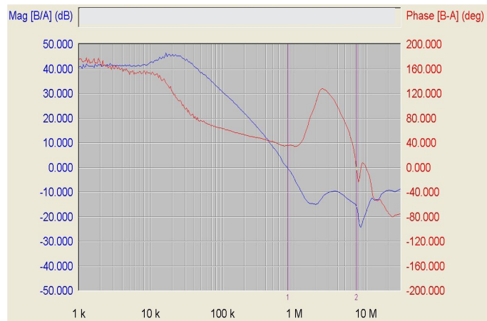
Figure 2 — Gain and Phase Bode Plot Fc = 810KHz, PM = 36 degree at 1A Source
