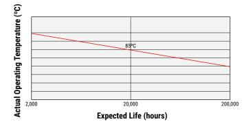
The effect of derating temperature can be seen in this graph.
