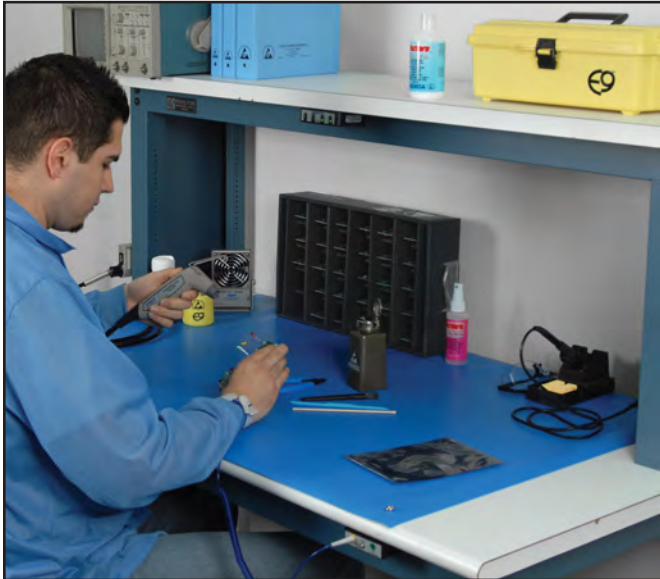
Figure 8: Using the Chargebuster Ion Gun
