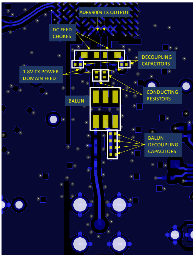
Figure 444. The Transmitter DC Chokes and Balun Feed Supply
