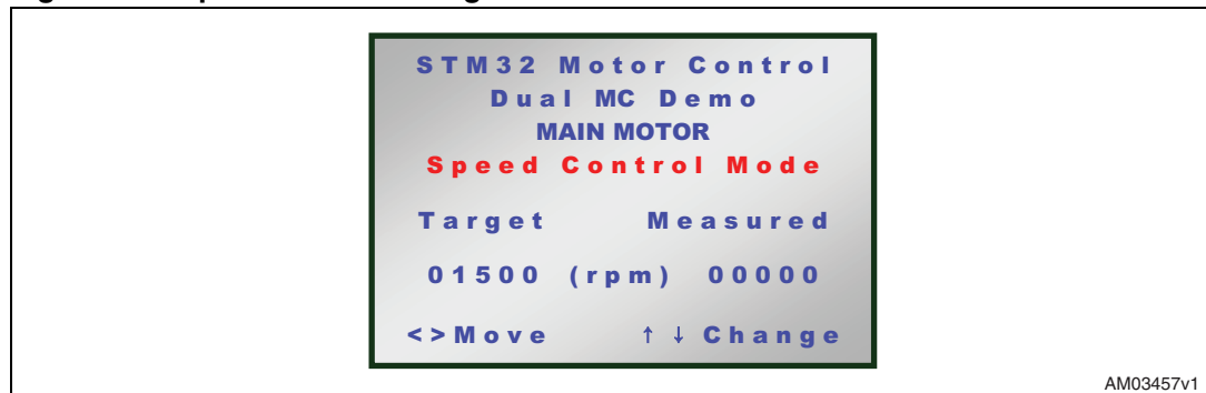
Figure 4. Speed control settings
