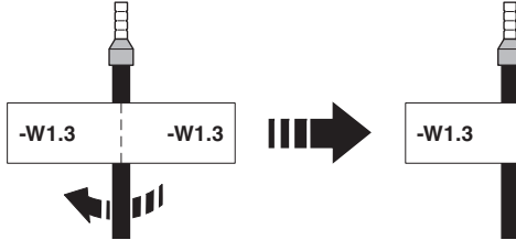
Figure 4-7 Example of a cable flag
