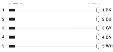
Contact assignment of 7/8" plugs/sockets
