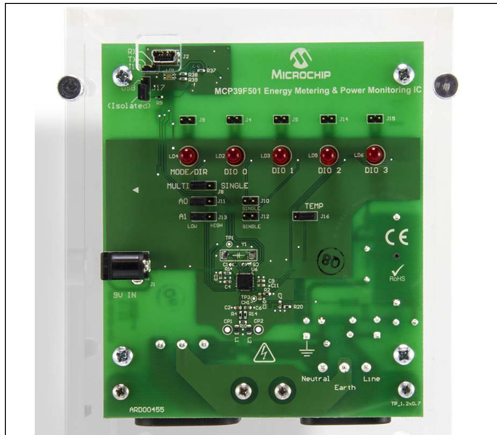
FIGURE 1-1: MCP39F501 Power Monitor Demonstration Board.
