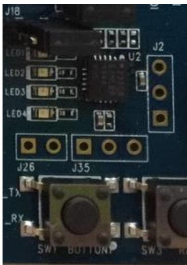
Figure 13: SPI IO Expander and connected Push button and LEDs
