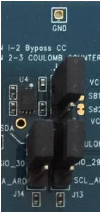
Figure 11: I2C sensor - Coulomb Counter
