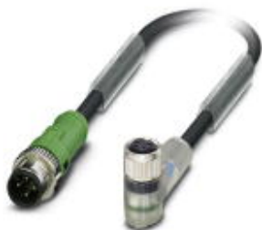
Sensor/actuator cable, 4-position, Variable cable type, Plug straight M12 SPEEDCON, A-coded, on Socket angled M8, with 2 LEDs, cable length: Free input (0.2 ... 40.0 m)
