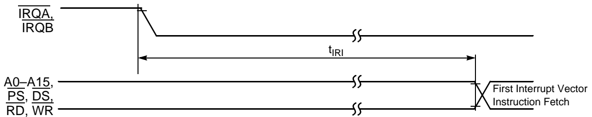
Figure 10-9 Interrupt from Wait State Timing
