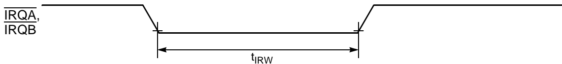
Figure 10-7 External Interrupt Timing (Negative Edge-Sensitive)
