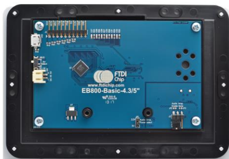
Figure 3-3 - VM800B module profile 5” display version
