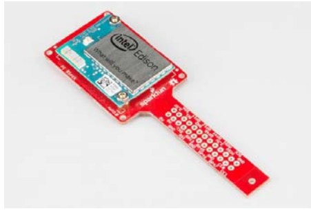
Edison installed on Pi Block
