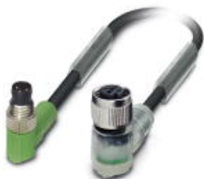
Sensor/actuator cable, 3-position, Variable cable type, Plug angled M8, on Socket angled M12 SPEEDCON, A-coded, with 2 LEDs, cable length: Free input (0.2 ... 40.0 m)
