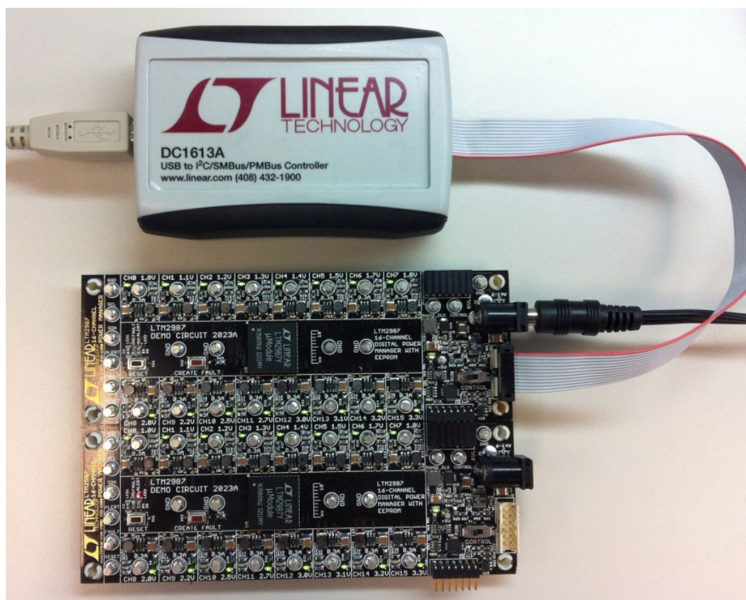
Figure 12. Array of Multiple DC2023A Demo Boards
