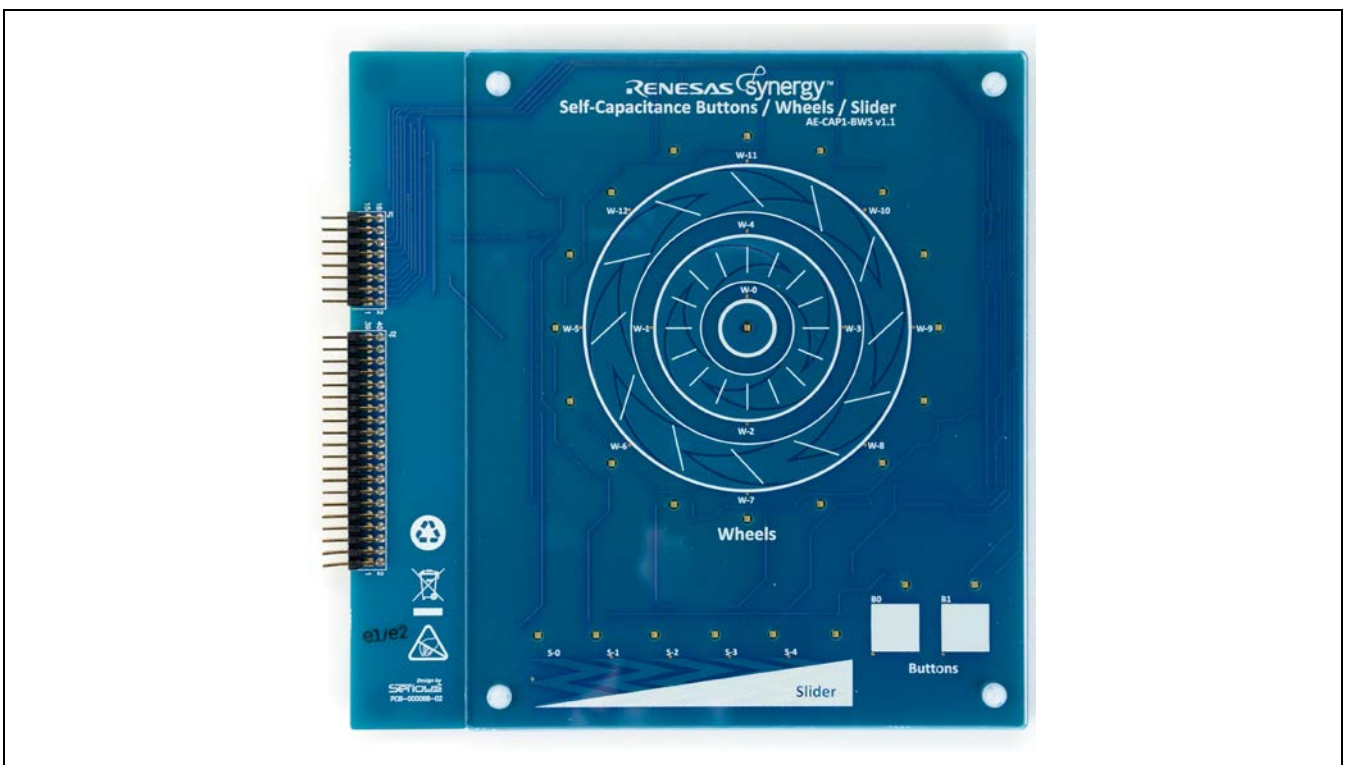
Figure 3 AE-CAP1-BWS Application Board
