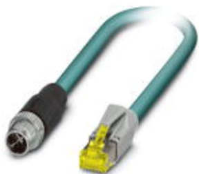
Network cable, Ethernet CAT6 A (10 Gbps), 8-position, PUR, water blue RAL 5021, Plug straight M12 SPEEDCON / IP65, coding: X, on Plug straight RJ45 / IP20, cable length: 20 m
