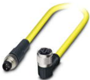
Sensor/Actuator cable, 3-position, PVC, Plug straight M8, on Socket angled M12 SPEEDCON, A-coded, Cable length: 0.5 m
