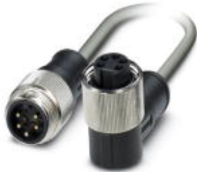
Bus system cable, DeviceNet, 5-position, PUR halogen-free, Gray RAL 7001, Plug straight 7/8"-16UNF, on Socket angled 7/8"-16UNF, Cable length: 2 m
