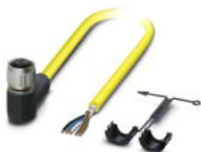
Sensor/Actuator cable, 5-position, PVC, yellow, shielded, free cable end, on Socket angled M12 SPEEDCON, A-coded, Cable length: 5 m
