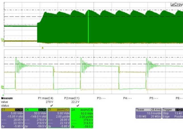
Figure 32. 85 V AC , AC Start at Full-Load (CH1: DET, CH3: Drain 1st )
