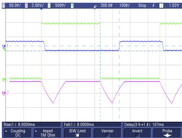
Figure 10, Soft-start with C_{SSCAP} = 10\text{nF} , V_{NC} = +50\text{mV} , V_{NO} = 0\text{V} Channel 1 = COM Channel 2 = SSCAP Channel 3 = IN
