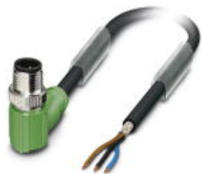
Sensor/actuator cable, 3-position, Variable cable type, shielded, Plug angled M12 SPEEDCON, A-coded, on free cable end, cable length: Free input (0.2 ... 40.0 m)
