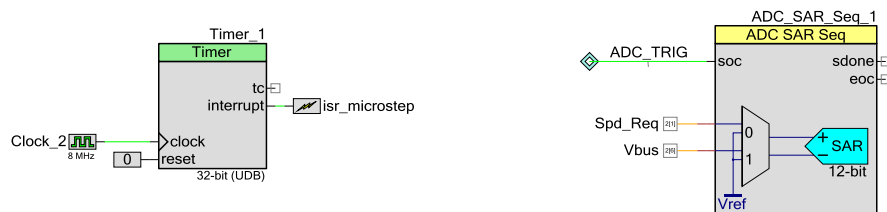
Figure 5-57. ADC,Button and Microstep Timer Schematic
