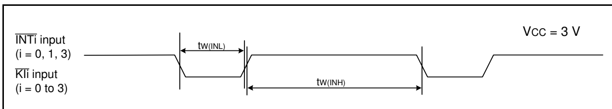
Figure 26.11 Input Timing for External Interrupt \overline{INTi} and Key Input Interrupt \overline{Kli} when Vcc = 3 V
