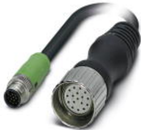
Sensor/Actuator cable, 17-position, PUR/PVC, Black RAL 9005, shielded, Plug straight M12-SPEEDCON, A-coded, on Socket straight M23, Cable length: 5 m
