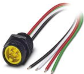
Flush-type connector, 4-position, Plug, straight, 7/8"-16UNF, on free cable end, Front mounting, with 1/2 inch-14 NPT mounting thread, Individual wires, cable length: 1 m
