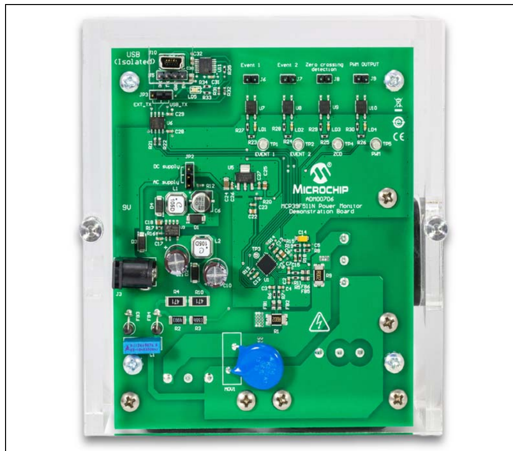
FIGURE 1-1: MCP39F511N Power Monitor Demonstration Board.
